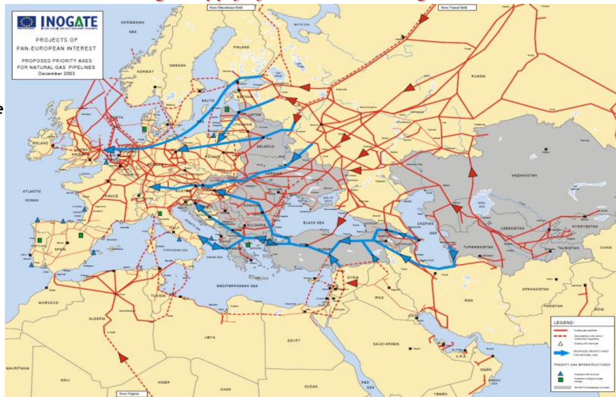
EU natural gas supply system and natural gas flow directions
